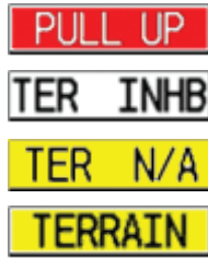
Figure 4-22 TAWS Annunciations from a 500W-series Unit
